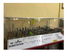
Working Prototype of 66/22 kV Outdoor type of Substation
