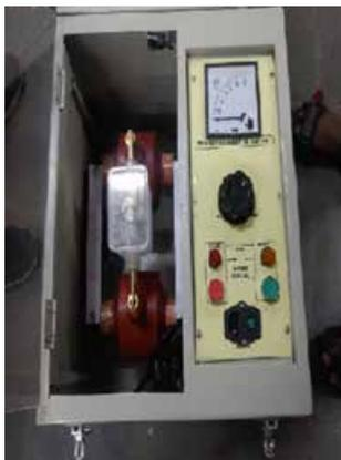
Transformer Oil Test Bench
